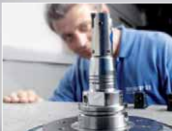
Wohlhaupter precision tools undergo standard balancing. They are precision balanced at the customer's request.
